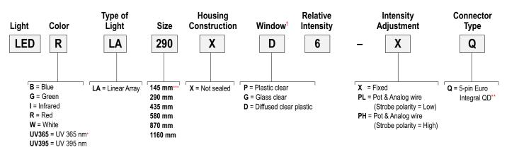
IP68 High-Intensity LED Linear Array Model Key, 24 V DC Example Model Number LEDRLA290AD6-XQ
