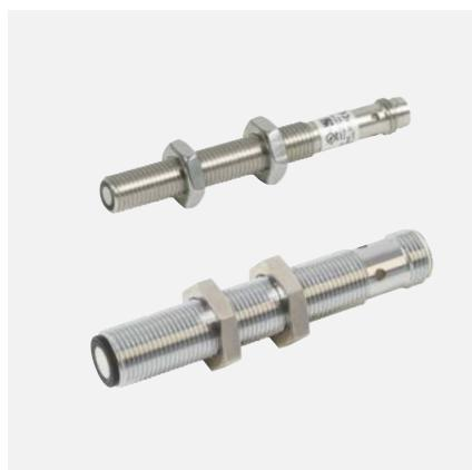
The smallest ultrasonic sensors in the M8 threaded housing are available in four versions, as screens or barriers, each with PNP or NPN interfaces. The sensors have a range of 100 millimeters and a blind zone of only 20 millimeters.
