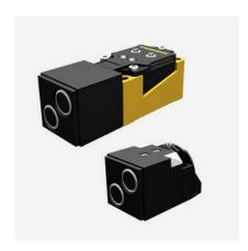
The rectangular CK40 with integrated connector or the CP40 variants with terminal chamber combine the advantages of a large detection range with a wide opening angle and a very small blind zone. These sensors are thus ideally suited for safe detection of objects that provide only a weak reflection signal due to their geometry or are moved in a large environment. Both the switching as well as the measuring devices can be customized easy to use via teach button.
