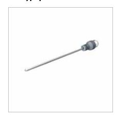
General data **Protection class** Connection IP67 male, M12 x 1 **Sensor quality** AISI 316L **Temperature operating** -50...500 °C range **Mechanical connection** for compression fer-Pressure resistance 100 bar rule fittings, protective tubing or direct mounting **Housing material** V4A (1.4404) **Outer diameter**  $3 \, \text{mm}$ t0.5 = 1.5 s/ t0.9 =Response time Class A **Accuracy** 6.0 s in water at 0.2 m/s
