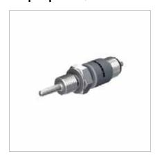
General data **Protection class** IP67 Connection male, M12 x 1 **Sensor quality** AISI 316L -50...120 °C **Temperature operating** range **Mechanical connection** G 1/8" male thread Pressure resistance 100 bar **Housing material** V4A (1.4404) **Outer diameter** 3 mm Response time t0.5 = 1.5 s/ t0.9 =Accuracy Class A 6.0 s in water at 0.2 m/s
