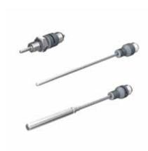
The core element of the TP series is a Pt 100 measuring resistor in 4-wire technology. All probes are connected to the processing unit via standard male M12 x 1.
