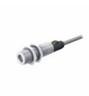
The non-contact sensors of the M18T series are mainly passive receivers. The thermal radiation of an object, normally between 8 and 14  $\mu$ m, is transformed into an electrical signal in a thermopile and then converted into an output signal. The D:S (distance: spot) ratio, which specifies the spot diameter at a defined distance, is important in this context. To monitor the surface temperature of the object optimally, the spot should be covered completely by the object.
