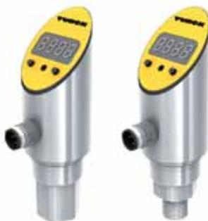
The PS300 series has been designed especially for hydraulic applications. The devices operate with a ceramic measuring cell. Available are versions with two switching outputs or one switching and one analog output. IO-Link communication is integrated as a standard. Highest process safety is achieved through a stainless steel housing, fully potted electronics and protection class IP69K.
