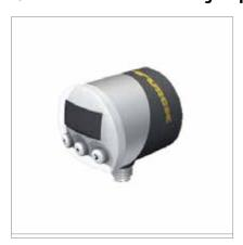
General data Output 1 switching output Output 2 switching output **Protection class** IP65 Connection male, M8 x 1 **Mechanical connection** NPT 1/8" male thread Medium temperature 0...50 ℃ Operating voltage 10.8...30 VDC **Housing material** AI/PVC **Switching frequency** 400 Hz **Accuracy switching** 1% v. E. BSL output
