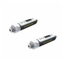
The PK-P pressure sensors operate with a silicon measuring cell. It is an open silicon chip with direct contact to the medium. The P version has a rotatable, cylindrical body with display. These sensors are only suitable for non-aggressive gas and compressed air applications. The processed signal is provided at the switching output.
