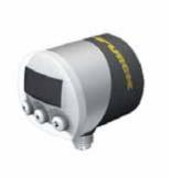
The PK-N pressure sensors operate with a silicon measuring cell. It is an open silicon chip with direct contact to the medium. The N version is manometershaped, features a display and a process connection on the back side. The processed signal is provided at the switching output. These sensors are only suitable for non-aggressive gas and compressed air applications.
