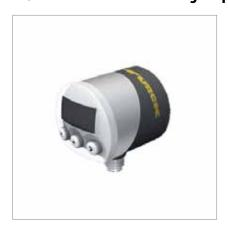
**General data** Output 1 switching output Output 2 switching output **Protection class** IP65 male, M8 x 1 Connection 0...50 °C **Mechanical connection Medium temperature** G 1/8" female thread Operating voltage 10.8...30 VDC **Housing material** AI/PVC **Switching frequency** 400 Hz **Accuracy switching** 1% v. E. BSL output
