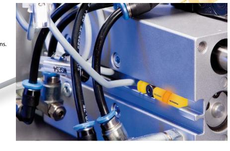
The 19.7 mm long BIM-UNTK is one of the most compact magnetic field sensors on the market. The active face is located at the sensor's end. This allows you to query the piston in the end position, even of small hydraulic
