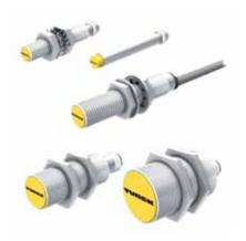
Typical applications for magnetic-inductive sensors include "pig" detection and gate monitoring. Since magnetic-inductive sensors are actuated by external magnetic fields, they achieve large switching distances despite their small size. In combination with the actuation magnet DMR31-15-5, the M12 sensors attain a rated switching distance of 90 mm.
