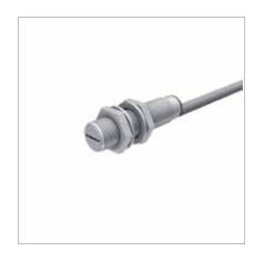
General data Connection 0.3 m Cable with con-Operating voltage 10...65 VDC nector, M12 x 1 Output **Switching distance** 2 mm, \_\_\_\_\_, 2-wire Operating current [mA] 100, 🛞 **Housing material** CuZn-T Ambient temperature 0...+70℃ **Dimensions** Ø 12 x 64 mm
