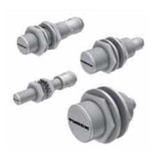
Harsh production environments of the automotive industry require *uprox*°+ sensors in PTFE-coated threaded barrels. The PTFE coating protects efficiently against weld splatter and drill cuttings. The non-ferrous coil system make the sensors resistant to strong magnetic fields.
