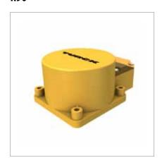
General data Operating voltage 10...65 VDC Output -, PNP **Switching distance** 100 mm, □ **Housing material** PBT Operating current [mA] 200, 🛞 **Ambient temperature** -30...+85 °C **Dimensions** 75 x 60 x 130 mm
