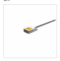
General data Operating voltage 10...30 VDC Output \_\_\_\_, PNP **Switching distance** 8 mm, 🚟 – **Housing material** GD-Zn Operating current [mA] 200, 🛞 **Ambient temperature** -25...+70 °C Dimensions 20 x 8 x 32 mm
