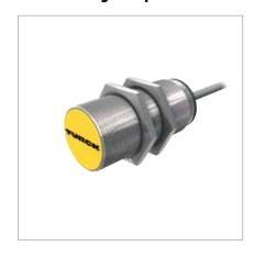
General data **Linearity deviation** 5 % of full scale **Measuring range** 2...10 mm Operating voltage 15...30 VDC Connection 2 m cable **Housing material** CuZn-Cr **Switching distance** Dimensions Ø 30 x 64 mm **Ambient temperature** -25...+70 °C Repeatability 1% of measuring range |A - B|
