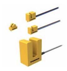
The slot sensors are U-shaped and the active face is located between the two arms. The sensor is activated when an object passes through the slot. Slot sensors detect laterally approaching targets reliably, regardless of their distance to the active face.
