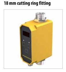
General data Medium liquids Connection male, M12 x 1 AISI 316Ti **Sensor quality** Pressure resistance 20 bar Medium temperature -10...90 ℃ Operating voltage 21...26 VDC **Housing material** PBT Function Inline sensor with in $tegrated\ processor$
