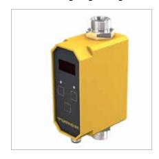
General data Medium liquids Connection male, M12 x 1 **Sensor quality** AISI 316Ti Pressure resistance 20 bar Medium temperature -10...90 °C Operating voltage 21...26 VDC **Housing material** PBT **Function** Inline sensor with integrated processor
