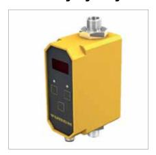
General data Medium liquids **Protection class** IP65 Connection male, M12 x 1 **Sensor quality** AISI 316Ti **Operating ranges** Flow Rate: 1...10 l/min **Mechanical connection** compression ferrule fittings for pipes Ø 10 x 1 (EN10305-1) Pressure resistance 20 bar Medium temperature -10...90°C Operating voltage 21...26 VDC **Housing material** PBT Inline sensor with integrat-**Function** ed processor
