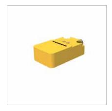
General data **Switching distance** 20 mm, **Housing material** PBT Ambient temperature -25...+70 ℃ **Dimensions** 40 x 20 x 68 mm Adjustment Potentiometer
