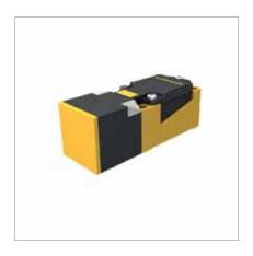
General data **Switching distance** 20 mm, **Housing material** PBT Ambient temperature -25...+70 °C **Dimensions** 40 x 40 x 114 mm Adjustment Potentiometer
