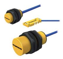
NAMUR sensors are approved for the zones 0 and 1. They are polarized 2-wire devices, changing their internal resistance in dependence on the attenuation (continuous linear/current characteristics). They can be connected to external switching amplifiers which convert current variations into binary output signals. The advantage: With an approved switching amplifier, they can be applied in Exareas as well as monitor wire-break and short-circuit continuously.
