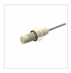
General data Connection 10...65 VDC 2 m cable Operating voltage Output **Switching distance** 7.5 mm, \_\_\_\_, PNP **Housing material PVDF** Operating current [mA] 200, 🛞 Dimensions Ø 18 x 74.5 mm Adjustment Potentiometer
