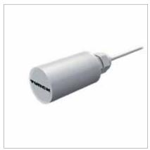
General data Connection 2 m cable Operating voltage 10...65 VDC Output \_\_\_\_, PNP **Switching distance** 20 mm, **Housing material PVDF** Operating current [mA] 200, 🛞 Ambient temperature -25...+70 °C **Dimensions** Ø 34 x 80 mm **Adjustment** Potentiometer
