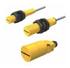
Cylindrically shaped capacitive sensors feature high switching distances and are available in many different designs. The standard types come in plastic housings and sizes from Ø 12 mm to Ø 40 mm, with connection cable, male or terminal chamber.
