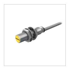
General data Operating voltage 10...30 VDC **Switching distance** 3 mm, **Housing material** Operating current [mA] 200, 🛞 CuZn, chrome-plated Ambient temperature -25...+70 °C Adjustment Potentiometer
