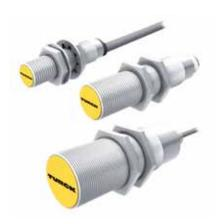
Cylindrically shaped capacitive sensors feature high switching distances and are available in many different designs. M12, M18 and M30 chrome-plated threaded barrels are available with connection cable or male connection. Besides the usual reliability, capacitive sensors feature standard properties such as automatic wetting compensation, excellent EMC and ESD properties and more flexibility with respect to mounting.
