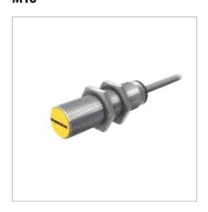
General data **Switching distance** 5 mm, **Housing material** CuZn, chrome-plated Ambient temperature -25...+70 °C
