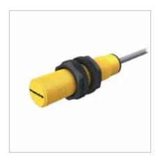
General data Operating voltage 10...65 VDC Output \_\_\_\_, PNP **Switching distance** 5 mm, **Housing material** PA12-GF30 Operating current [mA] **Ambient temperature** -25...+70°C 200, 🛞
