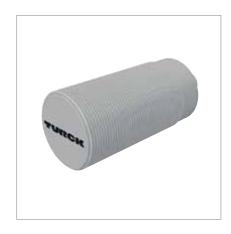
General data Connection male, M12 x 1 Operating voltage 10...65 VDC Output **Switching distance** 10 mm, \_\_\_\_, PNP **Housing material** LCP Operating current [mA] 200, 🛞 **Ambient temperature Dimensions** Ø 30 mm -25...+100  $^{\circ}$ C Adjustment Potentiometer
