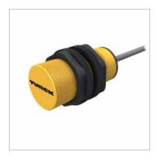
General data Operating voltage 10...65 VDC **Switching distance** 10 mm, **Housing material** PA12-GF30 Operating current [mA] 200, 🛞 Ambient temperature -25...+70 ℃ Adjustment Potentiometer
