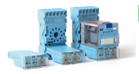
The modular timer system consists of individual plug-in timer modules with front cover, an 11-pole plug-in relay and a system socket with retaining spring.
