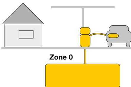
All equipment designed for use in zone 0 must meet category "ia" of equipment category 1 and must not contain any open switch contacts. Galvanic isolation between intrinsically safe and non-intrinsically safe equipment is recommended. If the intrinsically safe circuit has to be grounded for functional reasons, this must be implemented outside of zone 0, however, as close as possible to it. The devices must also be approved for gas group IIA, IIB and IIC.
