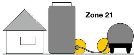
These can include areas in the close vicinity of filling or dust extraction stations, where dust deposits form and potentially explosive concentrations of flammable dust mixed with air may occur during normal operation.
