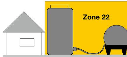
This includes areas in the vicinity of equipment containing dust which can escape due to leakage and where dust deposits can build up (e.g. mills from which dust is released and accumulates).
