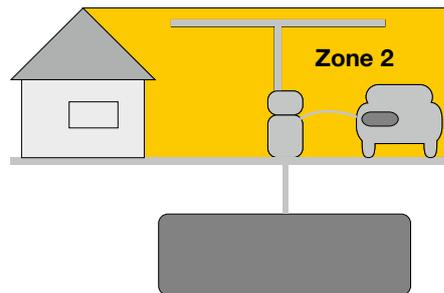
A test certificate from a test authority is not required for use in zone 2 as is compulsory in zone 0 and zone 1. Devices must comply with category 3. The equipment must meet the following criteria (EN 60079-15):
