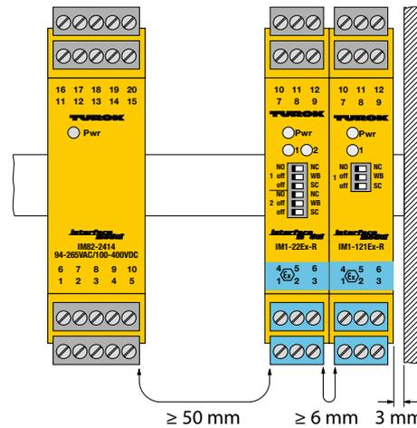
Either a partition must be used between intrinsically safe and non-intrinsically safe connections so that the minimum clearance is 50 mm (thread measure), or each connection must be covered individually and securely with a sleeve so that no part of the connection is exposed.
